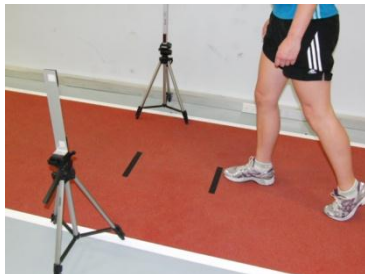
Figure 1 – the athlete starts the sprint with their toe on tape 50cm from start line.
